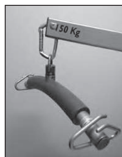
Correctly attached spreader bar.
