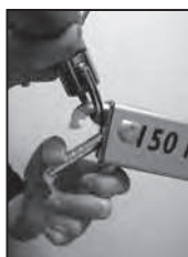
Easy opening of the carabineer by pushing the safety catch backwards with one finger and attachment of the spreader bar.
