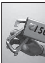
Carabineer correctly positioned on the lifting arm, ready for use.
